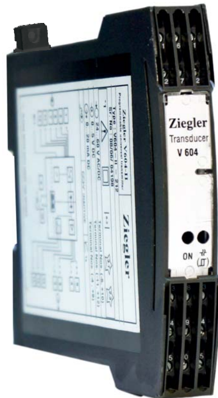
Fig2. Transmitter V604 in housing S17 screw hole mounting brackets pulled out.
