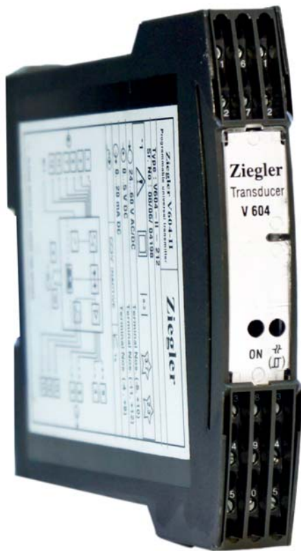
Fig1. Transmitter V604 in housing S17 clipped onto a top-hat rail
